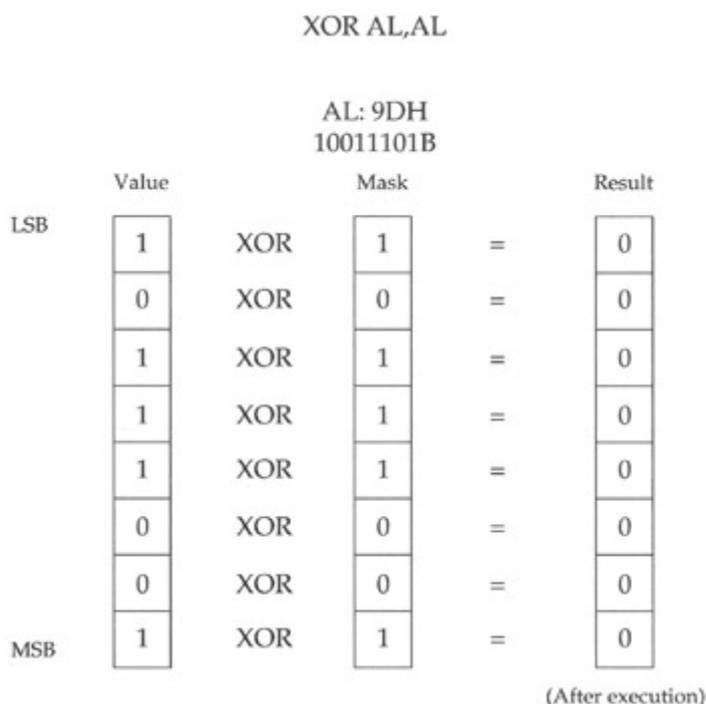
**Figure 10.3:** Using XOR to zero a register.
