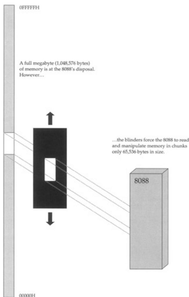
**Figure 6.3:** Seeing a megabyte through 64K blinders.
