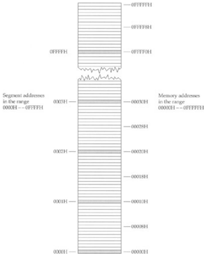
**Figure 6.4:** Memory addresses versus segment addresses.
