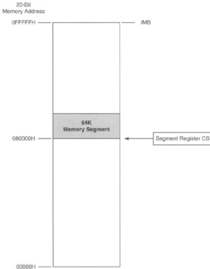
**Figure 6.2:** The 8080 memory model inside an 8086 memory system.
