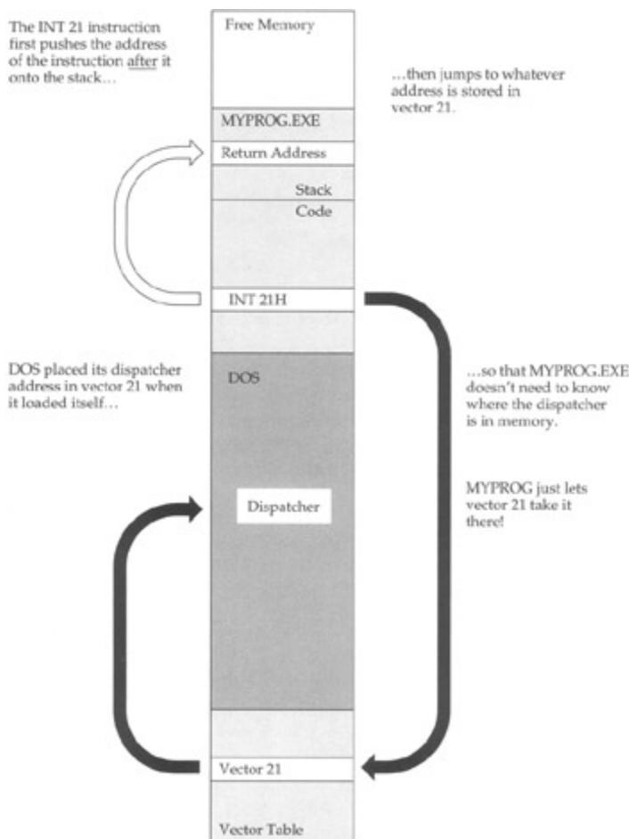
**Figure 8.4:** Riding the interrupt vector into DOS.
