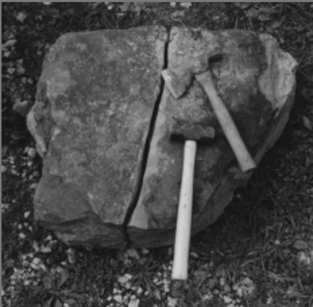
Left: This photo shows the two simple tools needed for cutting a stone. You can see the relatively clean cut with little or no flaking. Right: This photo shows a more jagged break. This can be caused by the physical makeup of the stone or by rushing and hitting the stone too hard.
