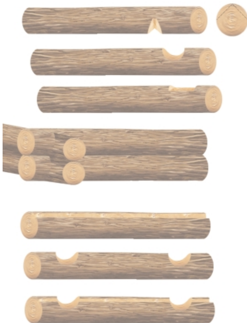
There are a variety of notches that can be used in building your log home.
