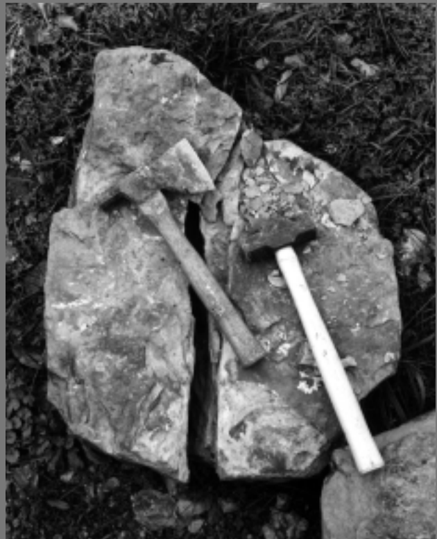
Left: This photo shows the two simple tools needed for cutting a stone. You can see the relatively clean cut with little or no flaking. Right: This photo shows a more jagged break. This can be caused by the physical makeup of the stone or by rushing and hitting the stone too hard.
