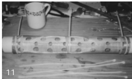
9. A hole-drilling template is wrapped around the 2-inch filter core.
