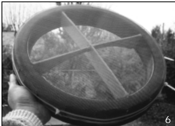
6. Plastic ties hold the brass screen to the lid.
