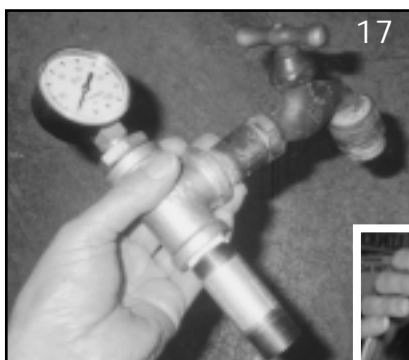
17. A pressure gauge and 3/4-inch drain valve are assembled, ready to be added to the pipe track.
