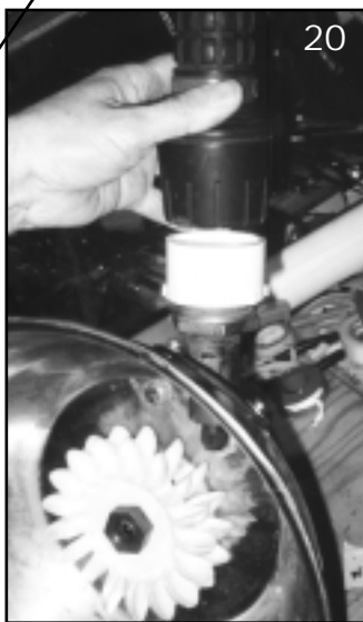
- Jet - Mounting plate - Pipe track coupler
