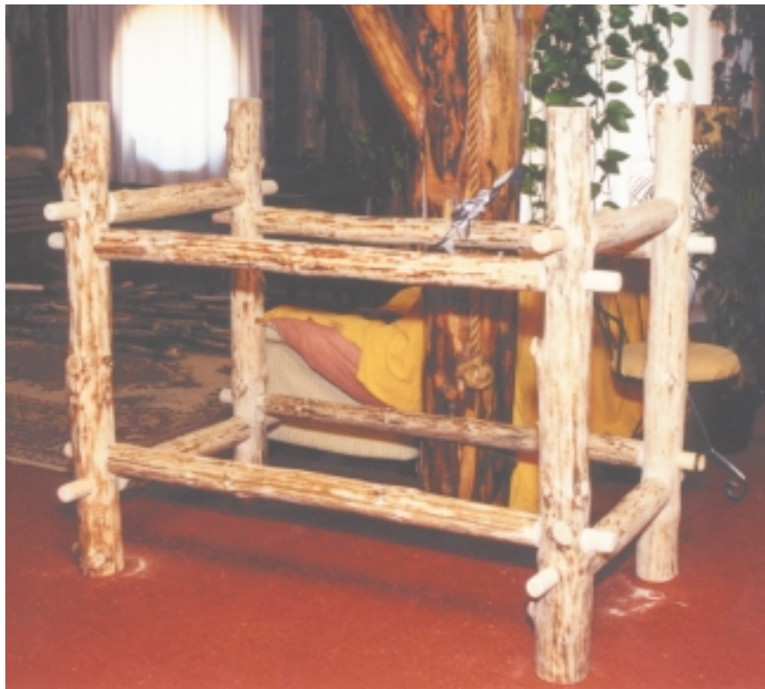
First assembly of frame to see if tenons slide easily into holes and also to check for plumb, level, and square, and to try mattress in the rectangle.
