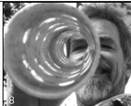
8. Inside view of the 2-inch filter core after drilling.
