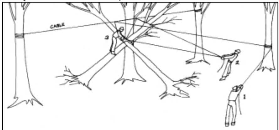
Rig for three-tree hang-up: helper number one keeps you from falling. Helper number two keeps your chainsaw from falling and services it as needed.
