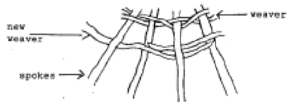
Figure 3. Sharpen the new weaver and insert.
