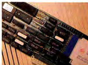
Cactus's board connects the II to a broadband network.
