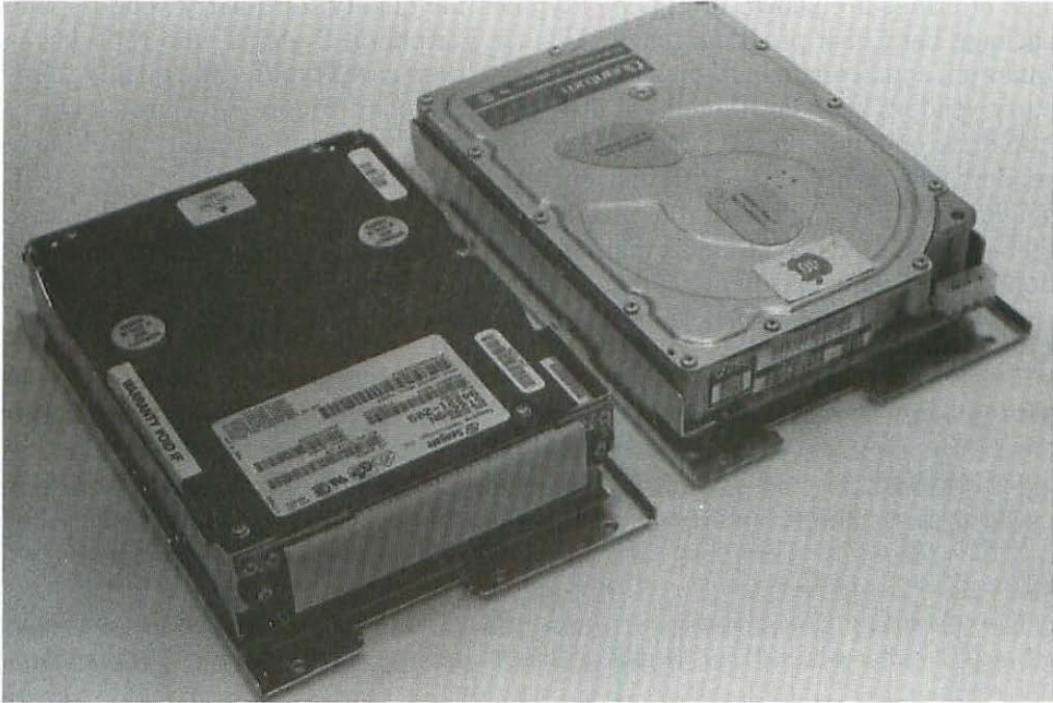
7-6 The Apple 160Mb Mac IIfx drive (left) and Apple 40Mb Mac II drive.
