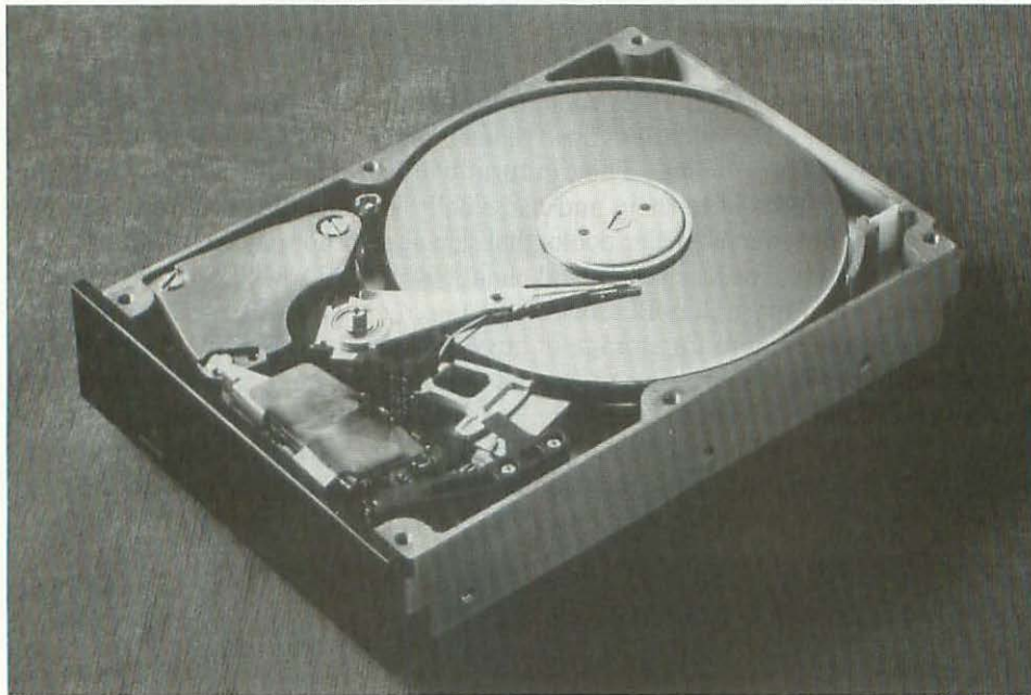
7-3 Prodrive LPS 52S/105S SCSI hard drive for the Macintosh.
