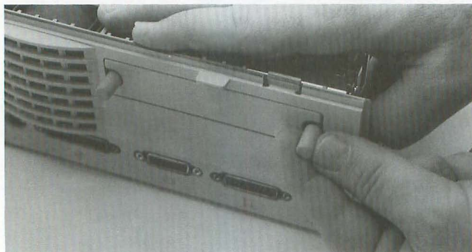
16-33 Reinstalling new Mac IIsi option cover so that the screws hold the adapter firmly in place.
