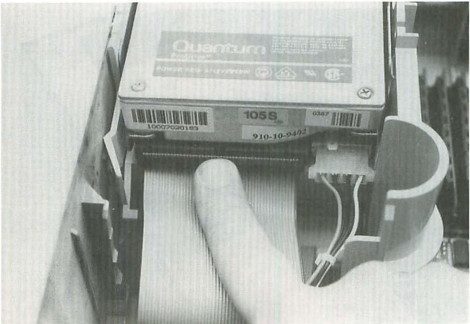
15-31 Detail of the Mac IIcx hard drive SCSI and power cable area.
