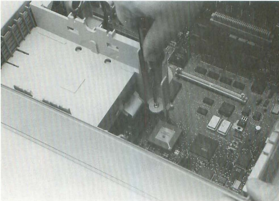
15-36 Remove the Mac IIcx plastic disk drive carrier holding screw.
