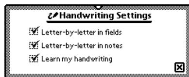
Letter-by-letter recognition controls the MessagePad's ability to recognize text that is not in its dictionary. If a word is not in the dictionary, the MessagePad uses letter-by-letter recognition to interpret the word. If letter-by-letter recognition is turned off (not checked) and the word is not in the dictionary, the MessagePad displays the word closest to it in the dictionary.
