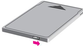
To unlock the card, slide the write-protection switch back toward the center of the card.
