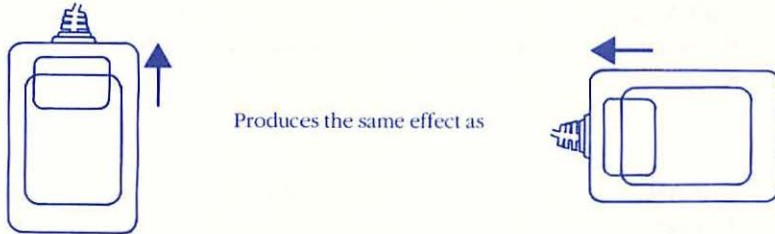
Mouse movements depend on the absolute orientation of the mouse.
