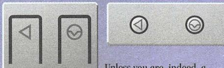
Unless you are, indeed, a programmer or knowledgeable about debuggers, the **Interrupt button** of the Programmer's Switch won't help you much. If you press it by mistake, just press the Restart button to re-boot the computer.
