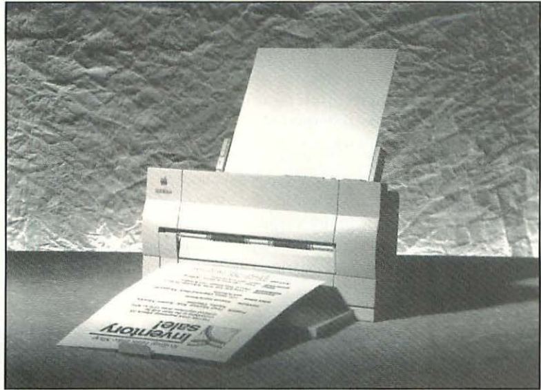
Figure 3.3: The Apple StyleWriter is Apple's lowest priced printer. Paper flows from top to bottom on this ink-jet printer. The StyleWriter is a QuickDraw printer, so you will probably want to use System 7 for TrueType fonts or Adobe Type Manager for PostScript fonts.
