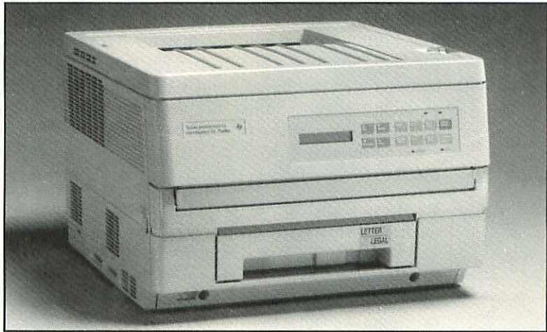
Figure 3.2: Texas Instruments makes a range of laser printers. The MicroLaser XL Turbo features an up-to-date specification, including PostScript Level 2, sixteen pages per minute, and a RISC processor.
