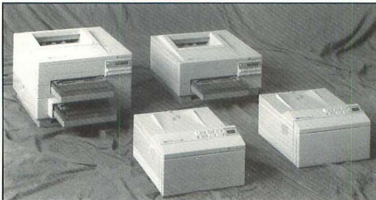
Figure 3.7: Here's a group of Hewlett-Packard laser printers. (Back, left to right) The LaserJet IIId and LaserJet III for printing eight pages a minute; (front, left to right) the LaserJet IIIP and IIP, which print at four pages a minute. You can buy these with the necessary AppleTalk interface and PostScript cartridge already installed.
