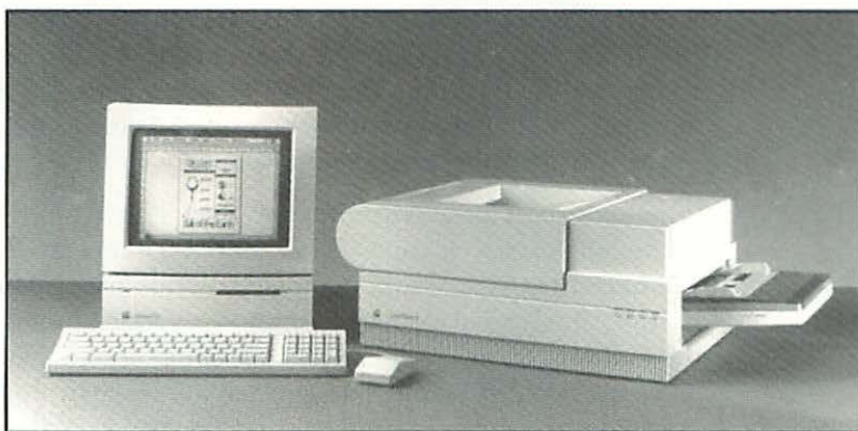
Figure 3.1: A Mac II and an Apple LaserWriter IIg. The LaserWriter has eight page per minute output and PostScript Level 2. Print and picture quality is enhanced by FinePrint, a resolution enhancement feature, and Photograde for better gray-scale images. The IIg also includes an EtherNet connector for network use.
