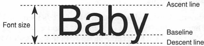
Figure 12-1. The size of a font is the distance between the tops of the tallest characters (the ascent line) and the bottoms of the lowest characters (the descent line).
