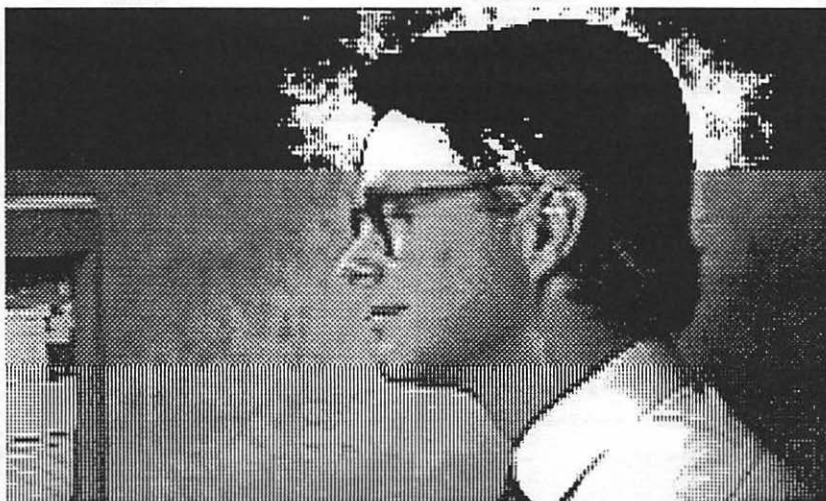
Figure 2.53. Three images are overlaid here. The top stripe has been "solarized" by clicking the Black and white button. The middle uses the standard values for a 300 DPI laser printer. The bottom uses the line screen with the angle set to 90 degrees.
