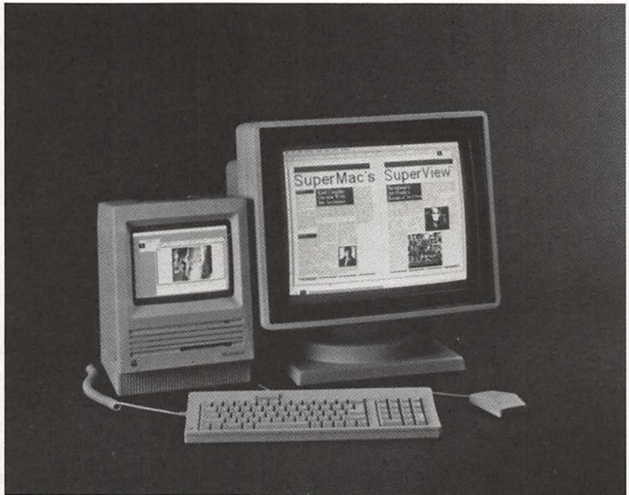
Figure 1-17. The SuperMac display card and large screen monitor for the Macintosh SE displays a complete PageMaker spread (2 pages), with readable (not greeked) 10-point type. If you perform screen-intensive tasks such as page makeup or drawing, a larger screen can offer a fast payback in comfort and increased productivity.
