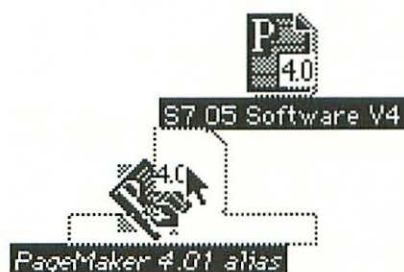
Figure 5.2: Application icons highlight when documents they can launch are dragged onto them.
