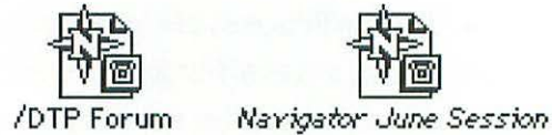
Figure 3.5: An original file and an alias of the file that's been renamed.
