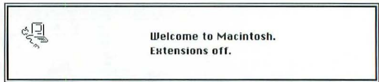
Figure 4.9: The Welcome to Macintosh dialog box as it appears when the shift key is pressed at startup.
