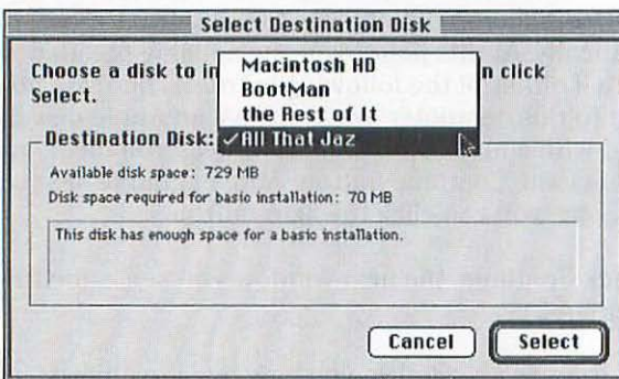
Figure A-4: If you have multiple hard disks, select the one you want to install Mac OS 7.6 onto from this pop-up menu.
