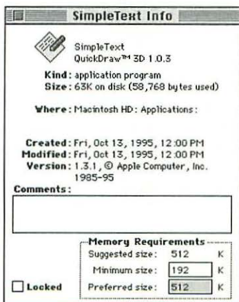
Figure 4-2: Reduce the Preferred size from 512K to a lower number (but not lower than the minimum size above it).
