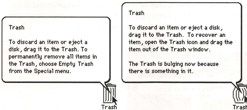
Figure 1-18. A balloon description can change depending on the state of an icon.
