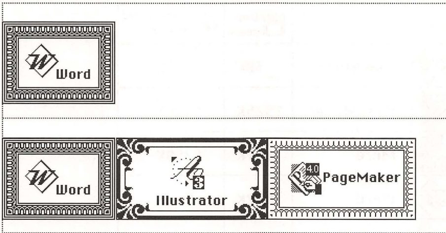
Figure 13-14. Quitting More and Illustrator and then reopening Illustrator gives it a partition next to Word and makes room for PageMaker.
