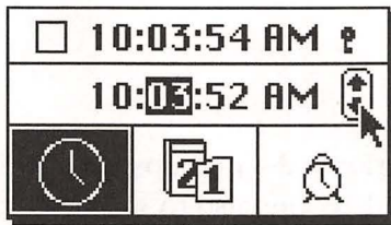
Figure 10-2. Change the time by selecting the numbers and using the arrows at the right of the edit area.
