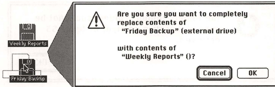
Figure 4-42. This alert checks with you before going ahead with a disk-to-disk copy; there's no drive listed for the second disk because it's not currently in a drive.
