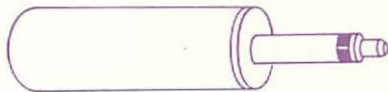
The audio-output port plug (Radio Shack #274-286). To silence the speaker, don't make any connections to the plug; merely insert the plug.
