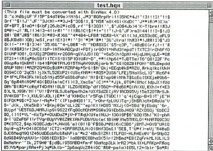
Figure 5-1: This is what a BinHex file looks like when you open it up in a text editor. Obviously, it will need to be decoded before it can be used.
