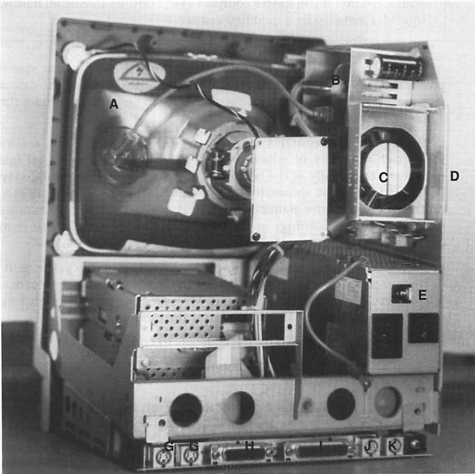
Figure 13-1: Inside a Mac SE. A: Video tube, B: Video, C: Fan, D: Analog board, E: Power supply, F: Logic board, G: ADB, H: External Floppy, I: SCSI, J: Printer port, K: Modem port, L: Audio out.
