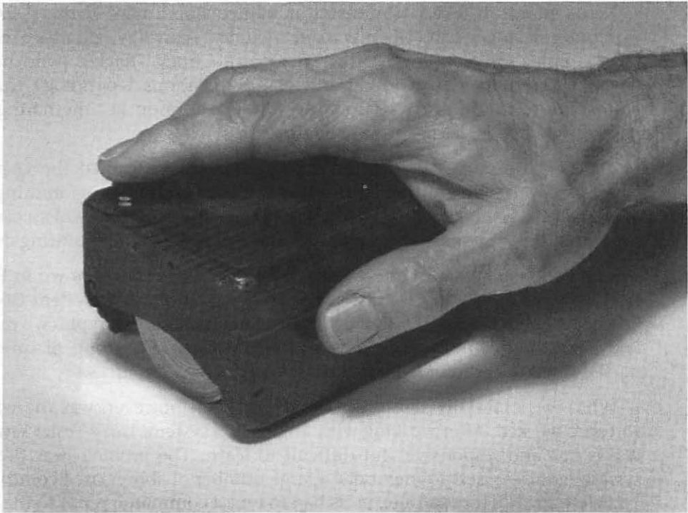
Figure 2-4. The first mouse: Douglas Englebart's "X-Y Position Indicator for a Display System" (photo courtesy of Douglas Englebart)
