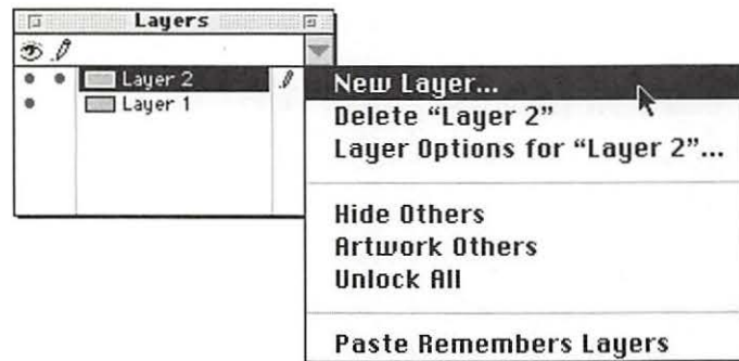
Figure 3.45 Create a new layer in Illustrator by clicking and dragging from the down-turned arrow in the Layers window.
