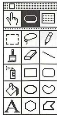
Figure 2.39 At the top of the HyperCard toolbox are tools you can use to select an element, create a button, or make a text box, and the other tools can be used to create and alter graphic elements and text.
