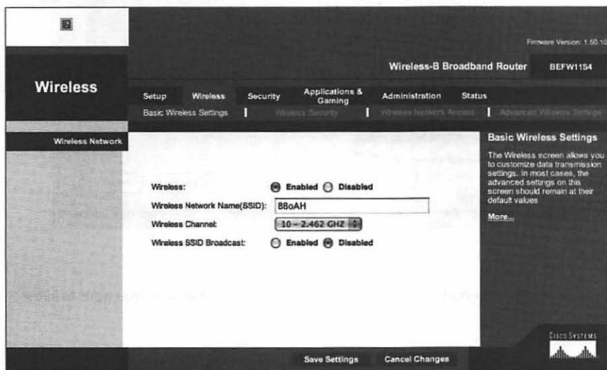
Figure 6-43. Turning off the SSID with a Linksys router
