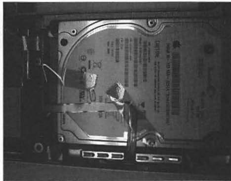
Figure 13-39. The hard drive that is being replaced
