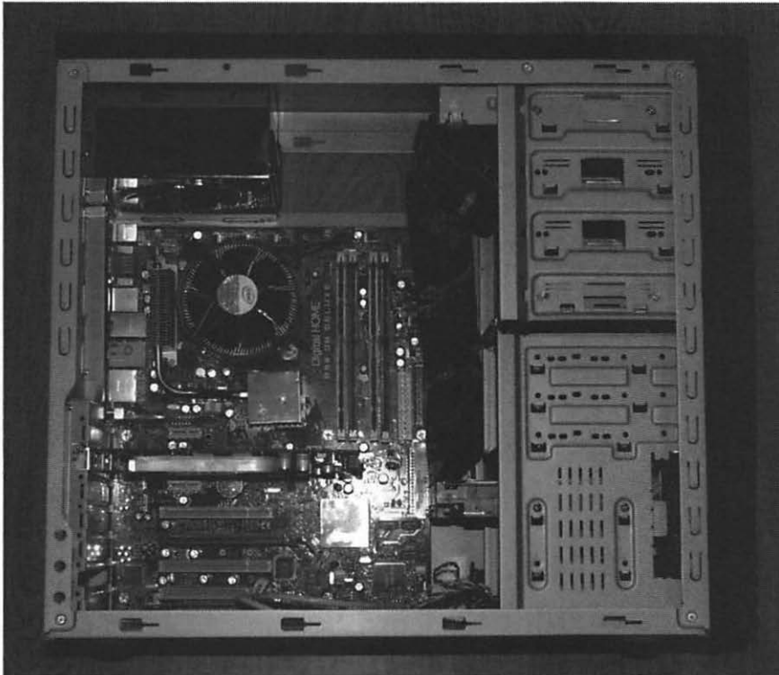
Figure 8-47. All of the components mounted in the case. Not much to it!
