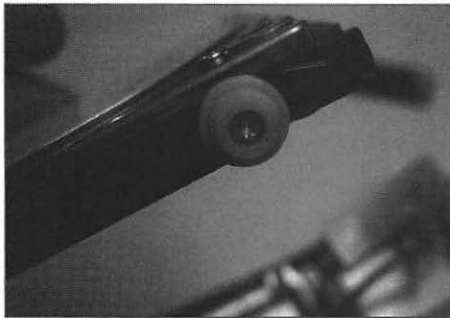
Figure 13-46. Swap the knobs from the old drive to the new drive
