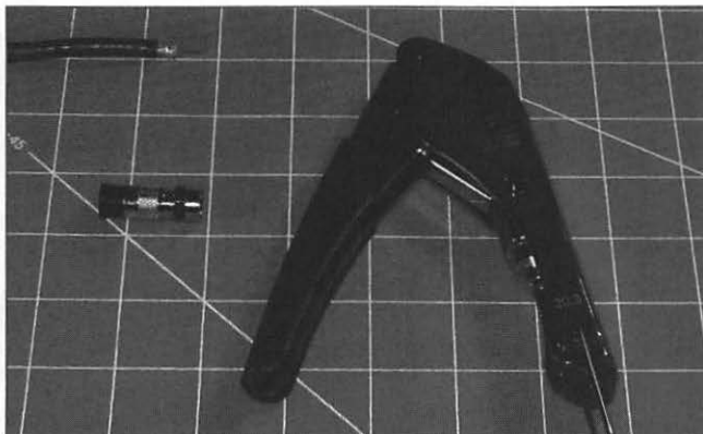
Figure 15-35. The cable, the compression fitting, and the compression tool
