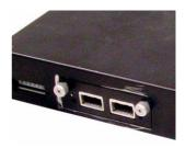
**6** Turn on the switch. The switch automatically detects the installed EM-422. Connect any necessary network cables to the EM-422 and check the LEDs to verify that it is functioning properly.
