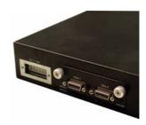
**6** Turn on the switch. The switch automatically detects the installed EM-412. Connect any necessary network cables to the EM-412 and check the LEDs to verify that it is functioning properly.
