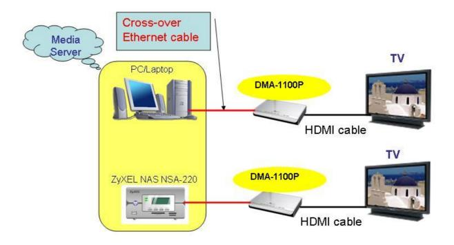
In this basic application scenario, you have the all devices including TV set, ZyXEL DMA-1100P, and PC/Laptop or NAS (with embedded media server) in the same room. Using DMA-1100P as media adapter and interconnect your PC or NSA with TV set. This is the simplest environment when deploy ZyXEL DMA-1100P.
