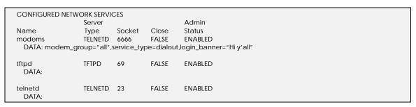
**3** TELNET to RAS1500's IP address with a TCP Port number matching the socket number set earlier.
