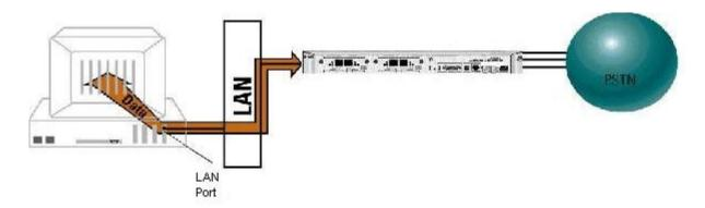
Modem Use of NCSI-Compliant Applications: Data Is Sent over the Network Directly to a RAS1500 Modem
