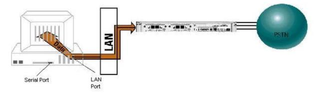
Modem Use of NCSIPort: Data Intended for Serial Port Is Redirected over the Network to a RAS1500 Modem
