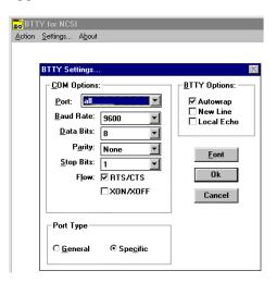
**3** You will be returned to the BTTY main menu. Click on <u>Action</u>, and <u>Connect</u> in the pop-up screen. When **OK** displays at the screen, you have successfully connected to RAS1500.
