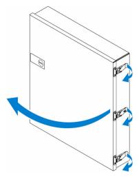
3. Place the enclosure on the wall-mount bracket, and align the tab on the back of the enclosure so that it fits into the notch on the wall bracket.
