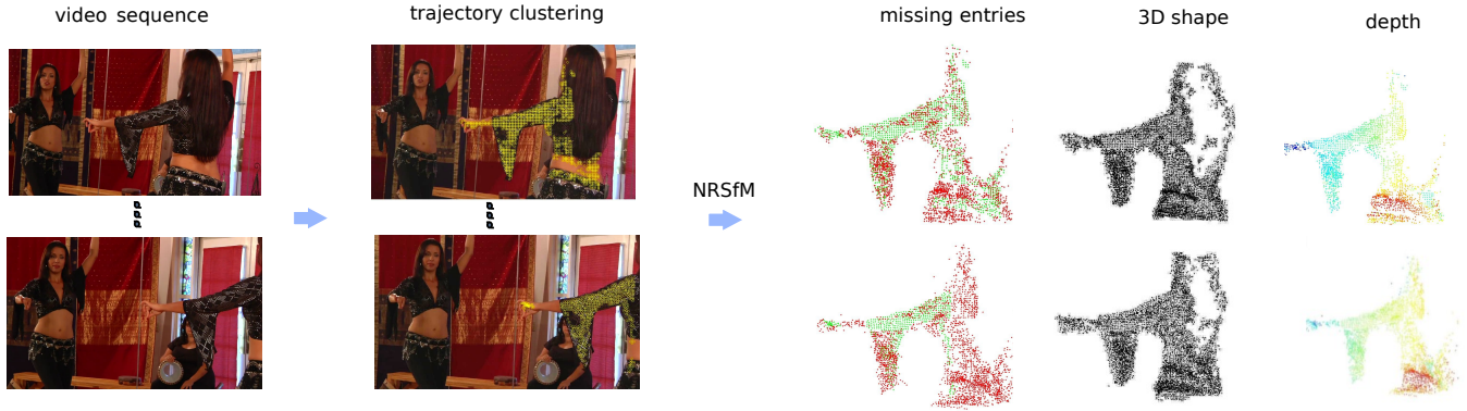
Fig. 16. Segmentation-based non-rigid structure from motion. Occluded trajectories on the belly dancer, that reside beyond the image border, are completed.
