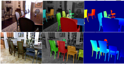
Fig. 19. Model Placement: Color image, placed models projected onto color image, depth map of rendered models (blue is closer, red is farther away).
