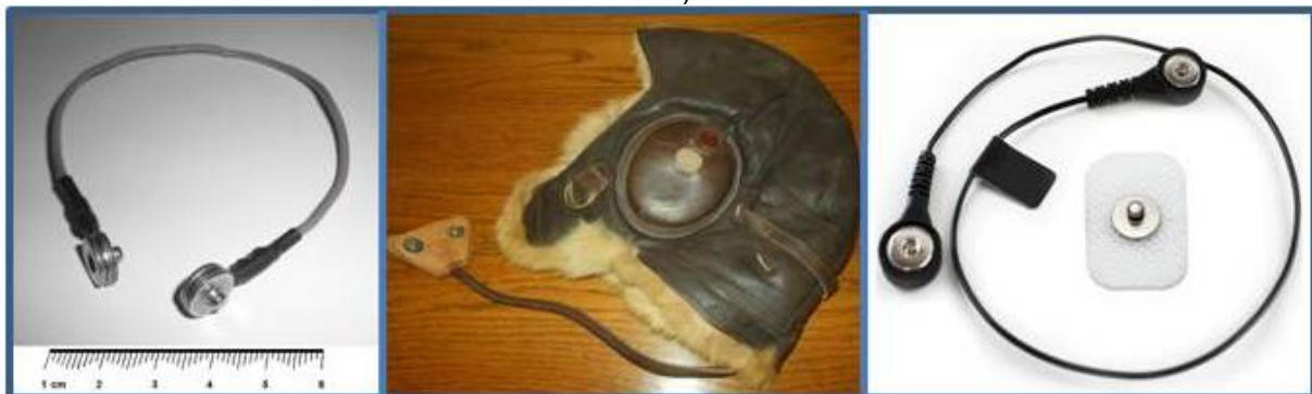
Figure 11. Electrical snap connectors. In 1921 J. d'Argaville Clark patented the first electrical connector utilizing snap fasteners attached to insulated wire (shown at left a later Nu-Way commercial version). They allowed quick and easy connections to low voltage power supplies and enabled experimental circuit boards to be built and modified rapidly. They were common in laboratories, schools and electronic design workshops up to the late 1960s. Cheap, brightly coloured, educational sets are still available today. Centre, a WWII Japanese electrically heated helmet, with a '+ / -' snap fastener connector for rapid attachment and disconnection to the aircraft's electrical system. Right, An important offshoot of Clark's idea is today's medical usage, with disposable stick on snap fastener backed electrodes, connected by leads to various monitors.
