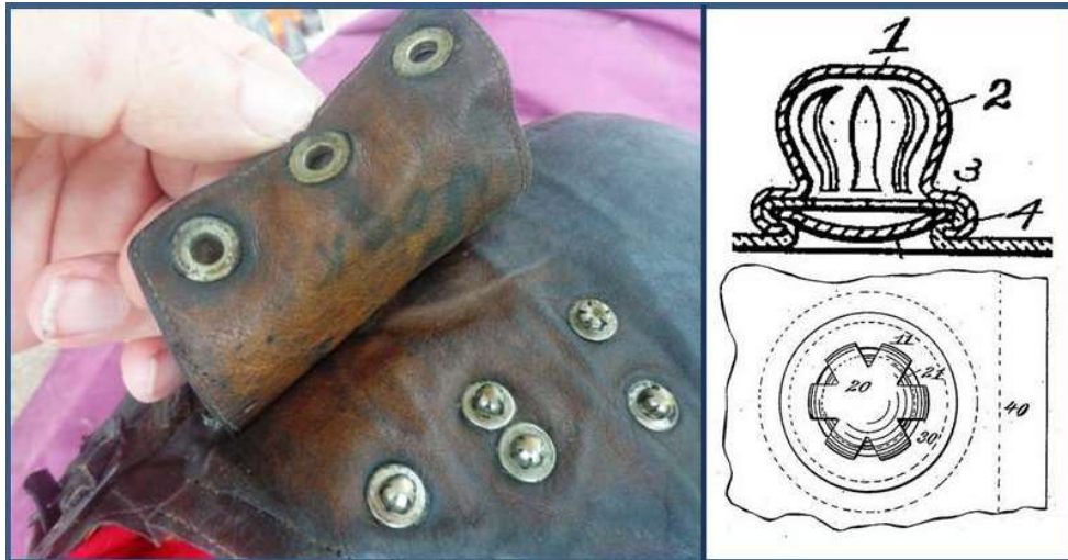
Figure 1. Left, Bird Cage snap fasteners on a 'cut down' Cowl Type RFC flying helmet, 1916-17. Right, patent drawings; bottom, the original design by P. A. Raymond, 1886, top 1902 – (first sighted use of the term 'Bird Cage'). The bird cage press stud was an example of a 'sprung clasp' snap fastener, in which the stud was a deformable clasp, which compressed as it entered the slightly constricted mouth of a rigid socket then expanded into the socket body.
