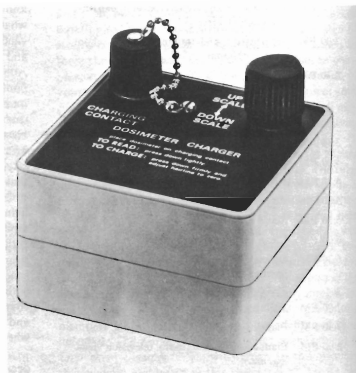
Individual radiation dosimeter and charger. This pen-like device gives a direct reading of personal radiation exposure. (Photograph courtesy of Nuclear Associates, Inc., 100 Voice Road, Carle Place, New York 11514.)
