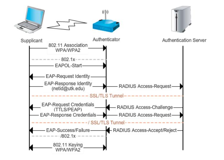
Until tunnel is established, AP is essentially an open access point
