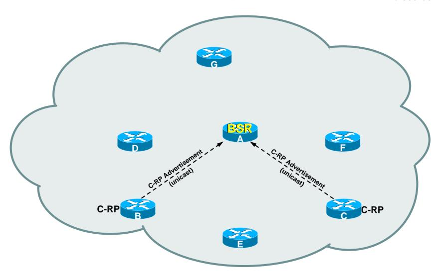
Cisco.com BSR BSR Msgs **BSR Msgs containing RP-set** Flooded Hop-by-Hop
