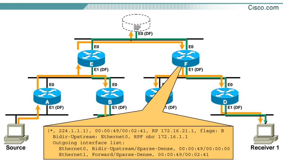
Router "F" forwards traffic on down the Shared Tree ala normal PIM-SM. RP doesn't even have to physically exist.
