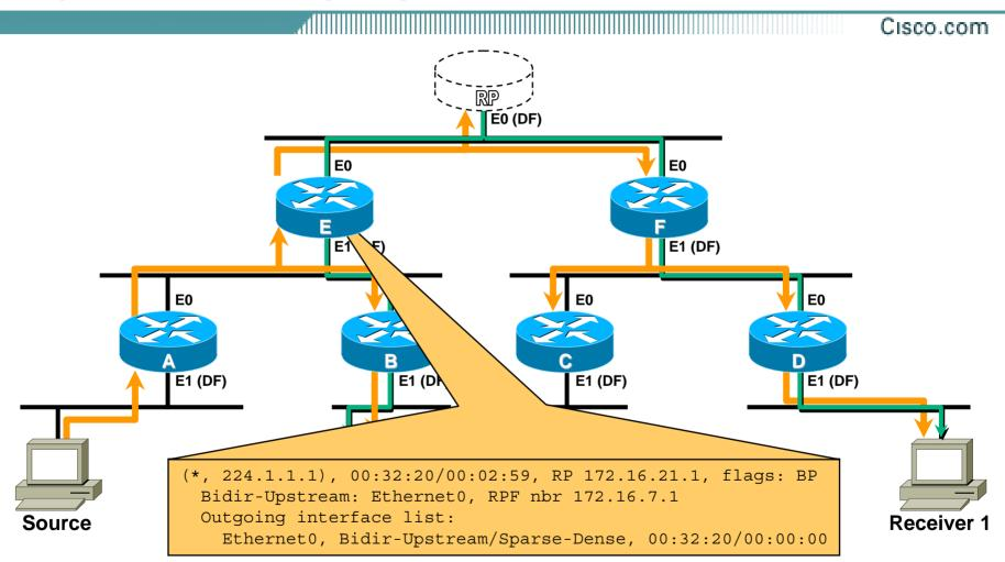
Router "E" forwards traffic onto core LAN segment.
