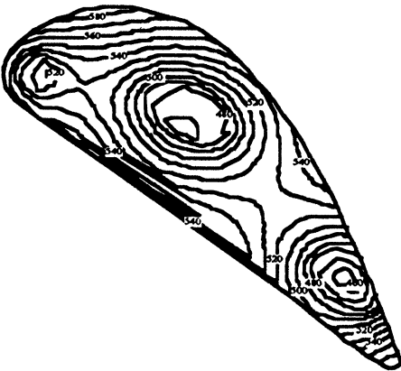
FIGURE 7(a) Temperature distribution for the reference blade.
