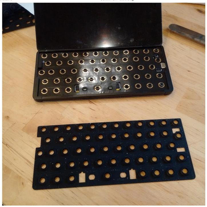
I'm surprised that the assembled faulty keyboards passed QA. But the silicone mats on their own are genuinely impossible to tell apart. It could be a question of material springiness or density, but I couldn't tell the difference and neither can my kitchen scales, hovering as they do, each, at precisely 9 grammes (and on subsequent weighins exactly 10 and sometimes 11).
