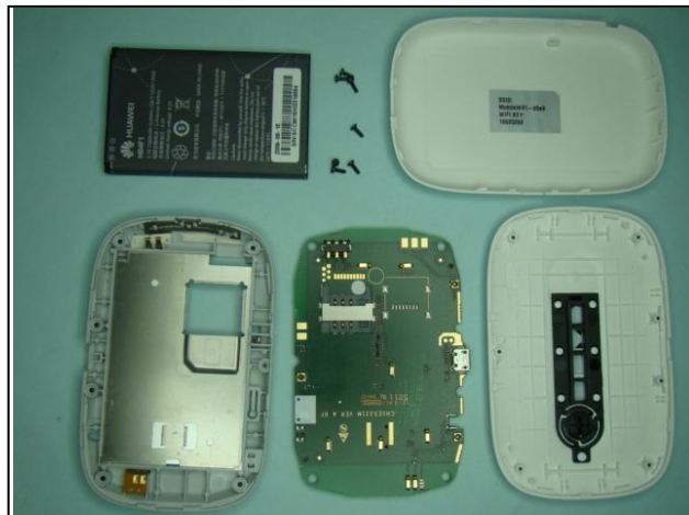
8. Disassembly procedure of the E5331 is completed.
