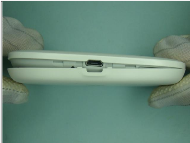
7. Install the battery cover.
