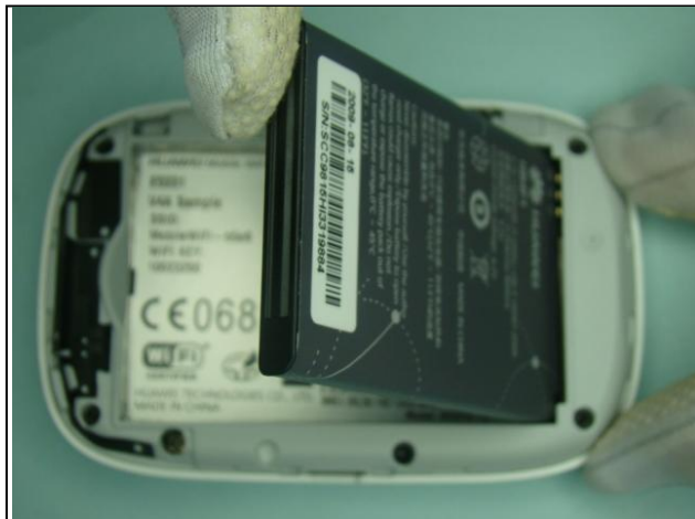
6. Install the battery.
